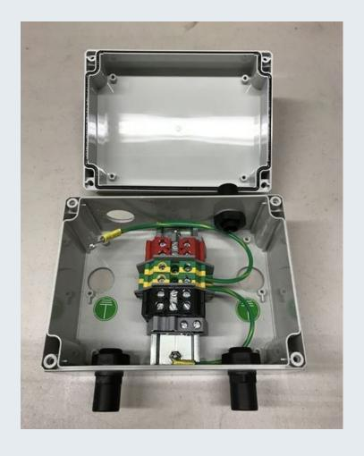
Afterward, the modified housing was integrated with the necessary components and subassemblies, including custom gaskets, cable glands, and DIN rail terminal blocks. The assembly team utilized custom-developed tooling and fixtures to optimize the accuracy and speed of the assembly operation, combined with quality assurance analytics to ensure the product met the required specifications and standards. This ensured the customer received the products they needed when they needed them.
